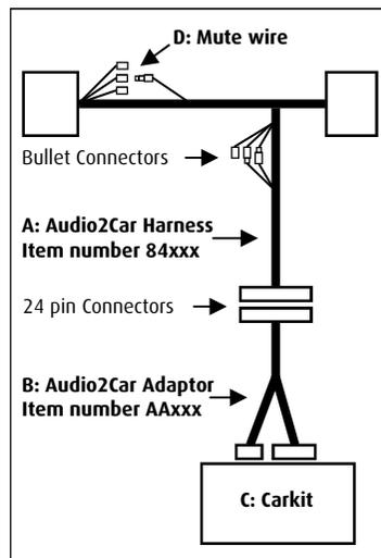
Audio2Car harness between the connector and radio / amplifier unit. **Note:** Some radios may require a security code to be entered after the power connectors have been removed.
